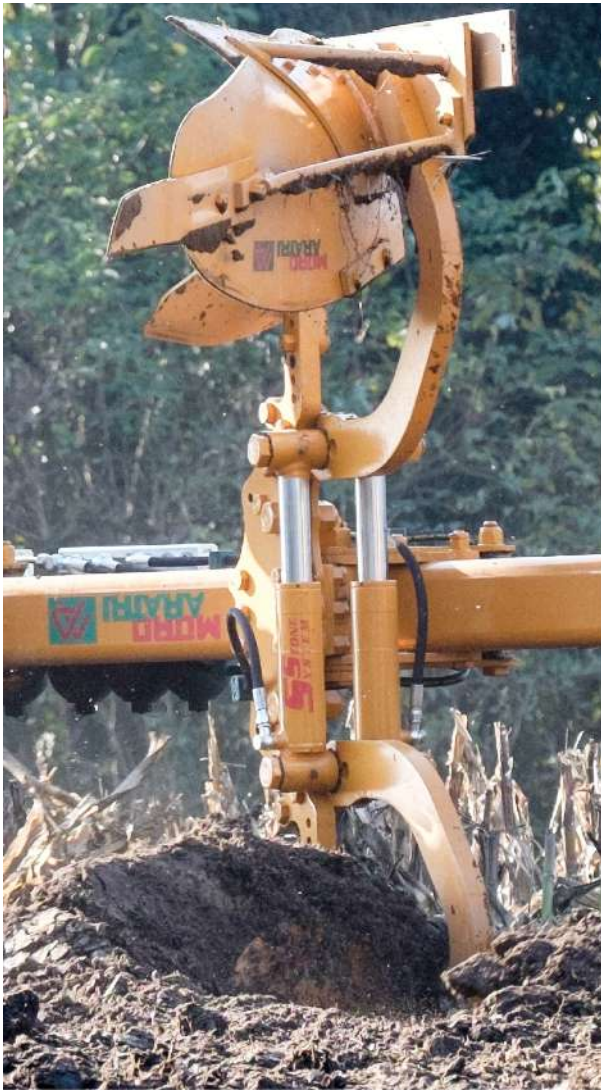
STONE SYSTEM element in working position and in simulation of obstacle
